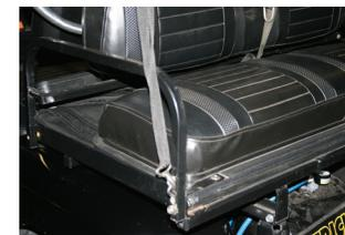
3. Install frame (with cloth cover and straps pre-assembled at the factory) by holding frame upright and sliding hinge bolts into the seat back support holes as shown. Be sure to slide the basket (if applicable) onto the bolts before assembling the washer and locknut. Important Note: Tighten all new hardware securely!
